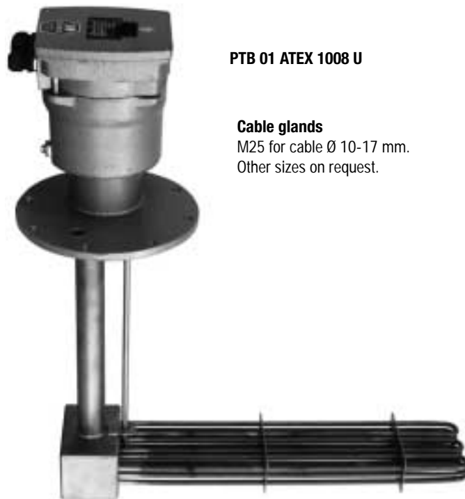
L-shaped immersion heater 4,5kW Type DHF-4,5-T6
